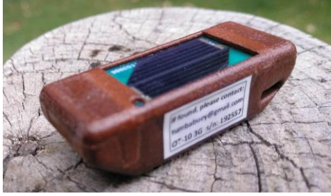
Figure 6. GPS transmitter OrniTrack-10, used for tracking Sacapuntas, Compás and Botellín. Source: Tumbabuey ringing group
